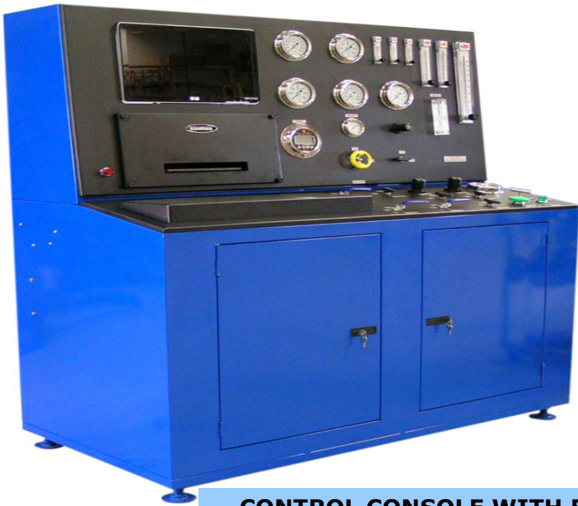
CONTROL CONSOLE WITH FLOW METERS AND DATA ACQUISITION SYSTEM
