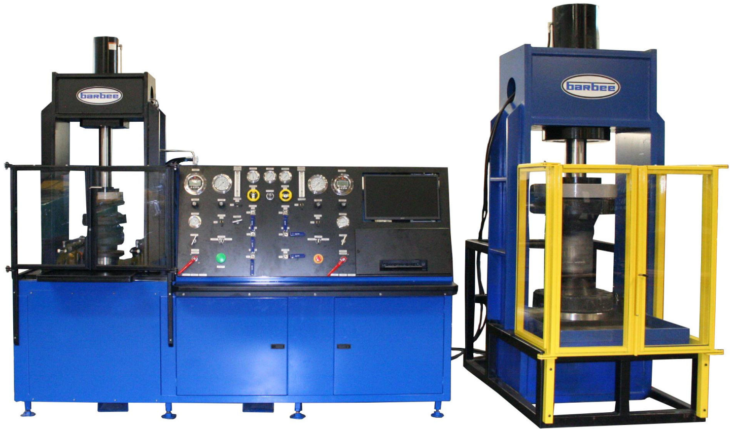
LVR MODEL SHOWN WITH A DUAL STATION: 100 TON CLAMPING FIXTURE ON THE CABINET AND A 400 TON FREE-STANDING FIXTURE FOR LARGER VALVES. DUAL INDEPENDENT HYDRAULIC AND HYDROSTATIC TEST SYSTEM.
